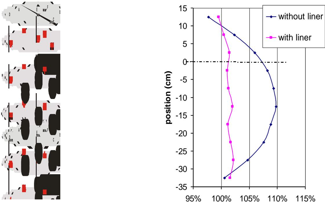
Fig. 3. Si ingot equipped with Al:Au(2%) neutron flux monitors and measured neutron flux density profile with and without Ni-liner.
