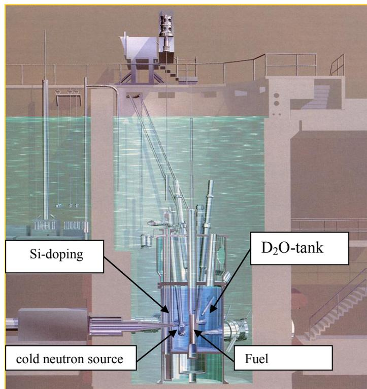
Fig. 1. Conceptual design of the FRM II moderator tank with some key components indicated.
